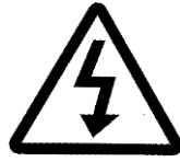
Danger!: High Voltage
